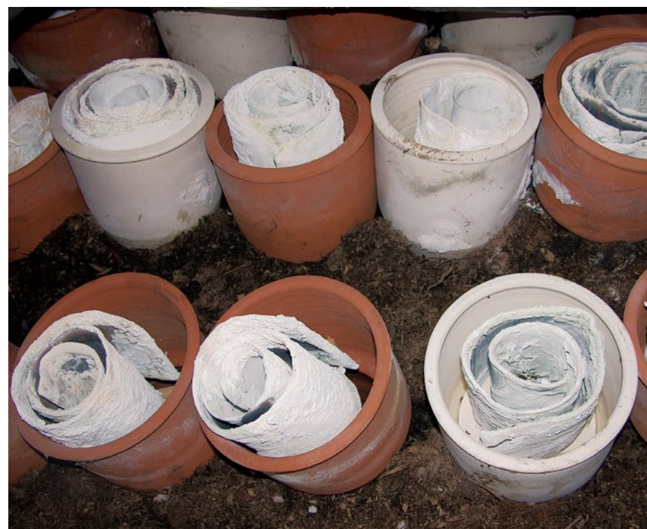
In this image, rolls of lead corrode in the "stack process" or Old Dutch method of making the pigment lead white. This lead has been exposed to acetic acid vapor, moisture, and carbon dioxide produced from fermented matter such as horse manure, which also provides heat. These together cause the lead to corrode, producing scales of lead (flake white).
