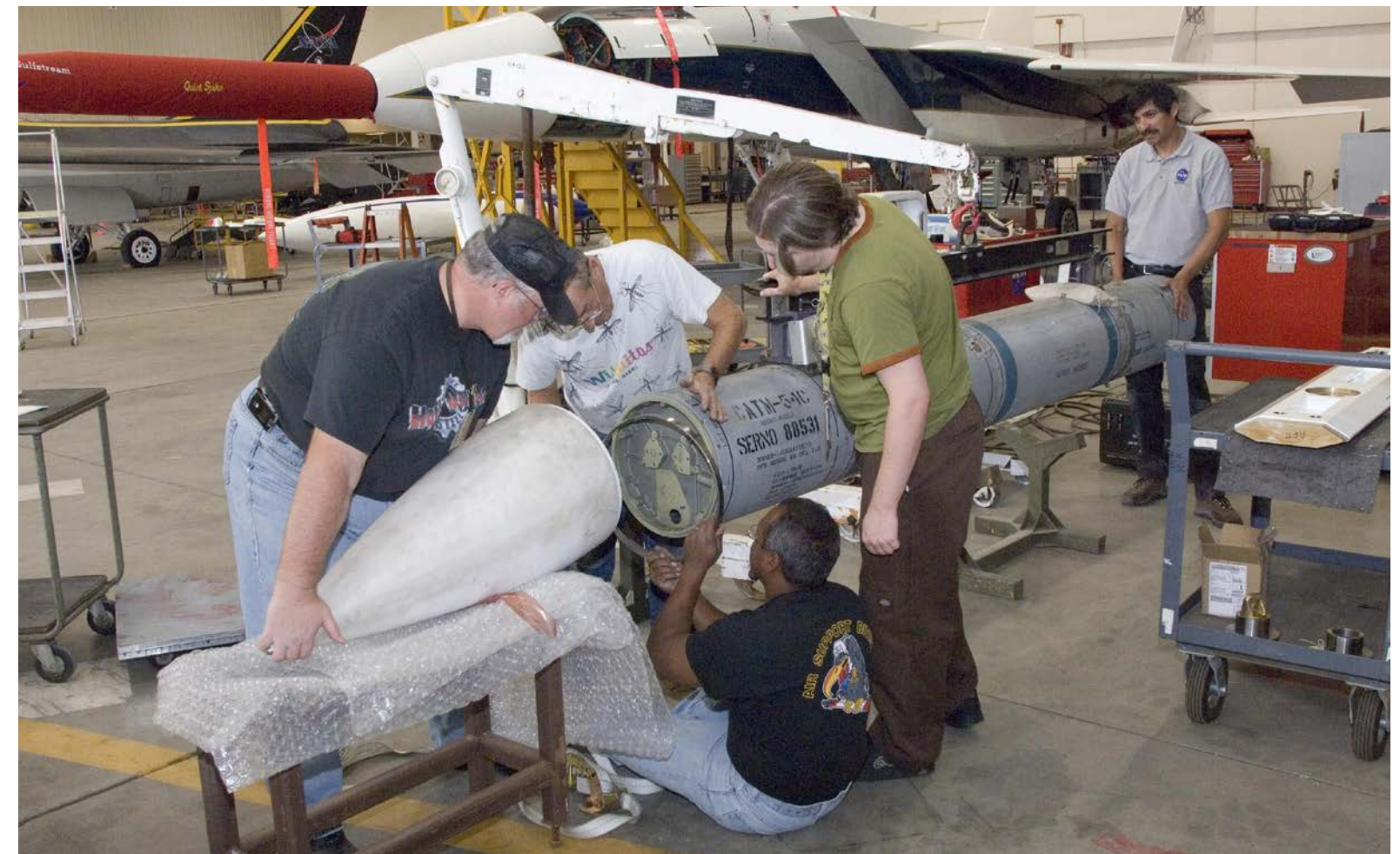
NASA Dryden aircraft and avionics technicians install the nose cone on a hypersonic Phoenix missile prior to a fit check, in this file photo.
