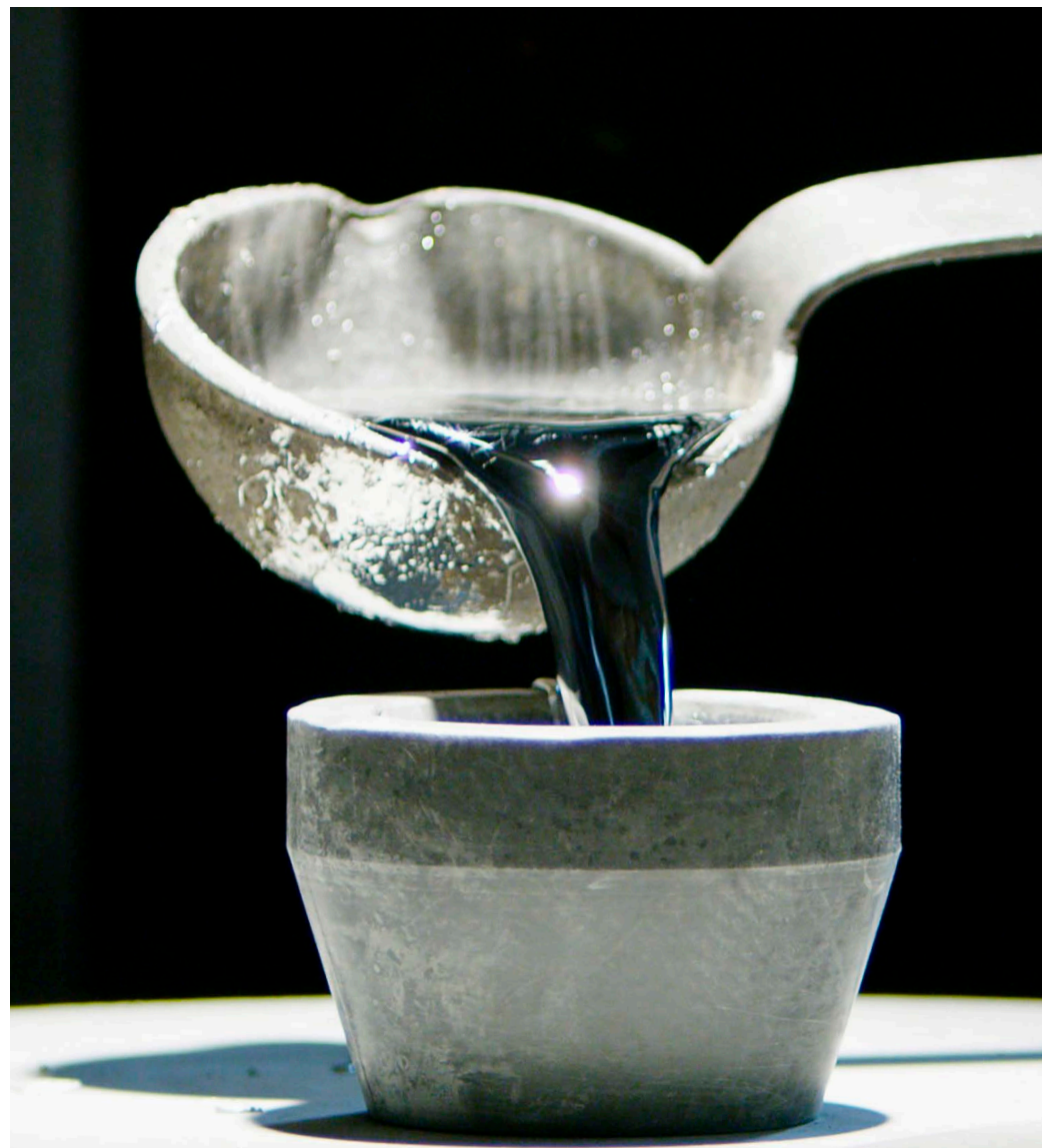
(Above) Molten pewter being poured into a cast.
