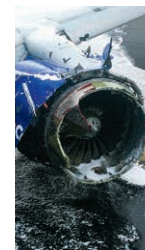
The damaged engine from Flight 1380.
