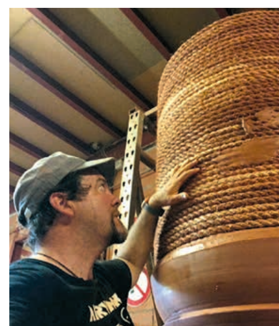
Clay is applied directly to the rope in order to shape the pot.
