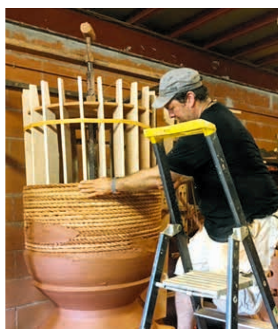
Yannick Fourbet carefully wraps sisal rope around the plywood frame.
